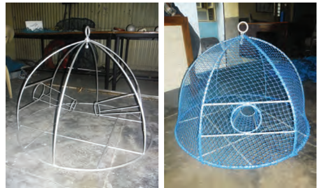
Fig.1. Various stage of fabrication of trap
