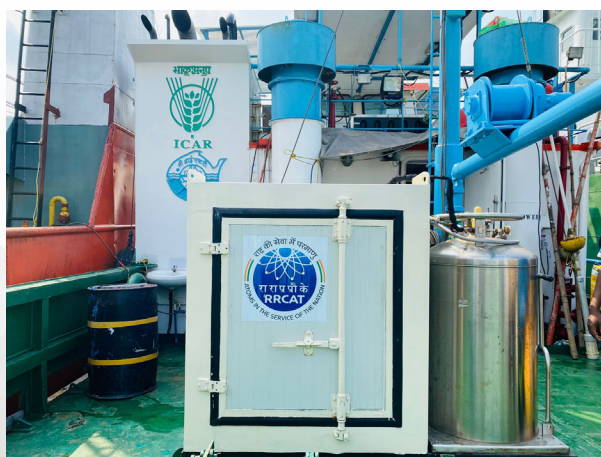
Figure 1. Liquid nitrogen chiller installed in the ICAR-CIFT fishing vessel
