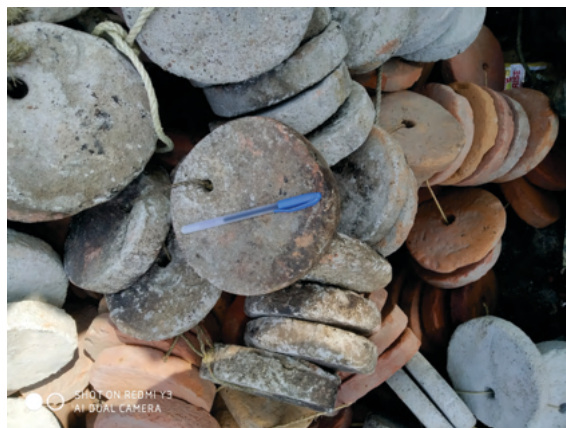
Fig.1 and 2 Sinkers made of concrete and stone
