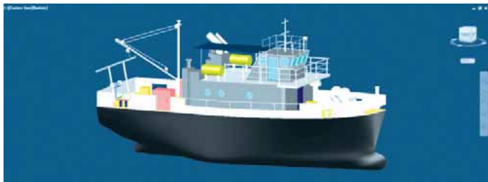
3D design of 19.75 m L_{OA} combination fishing vessel
