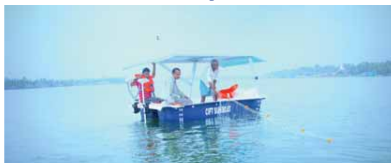
Multi purpose solar powered FRP boat in operation
