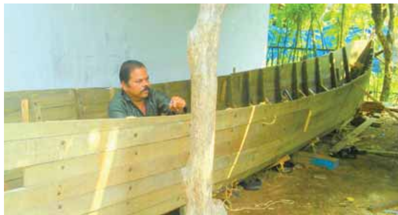
Coconut wood canoe under construction
