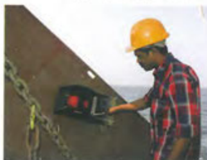
ITI sensors fixed to the otter boards for horizontal opening
