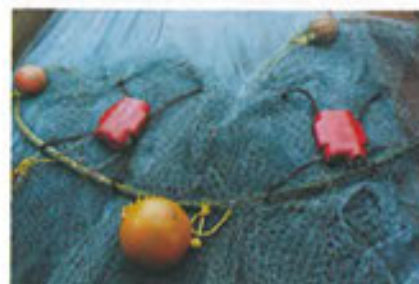
ITI sensors tied to the head rope of trawl for vertical opening and depth profile
