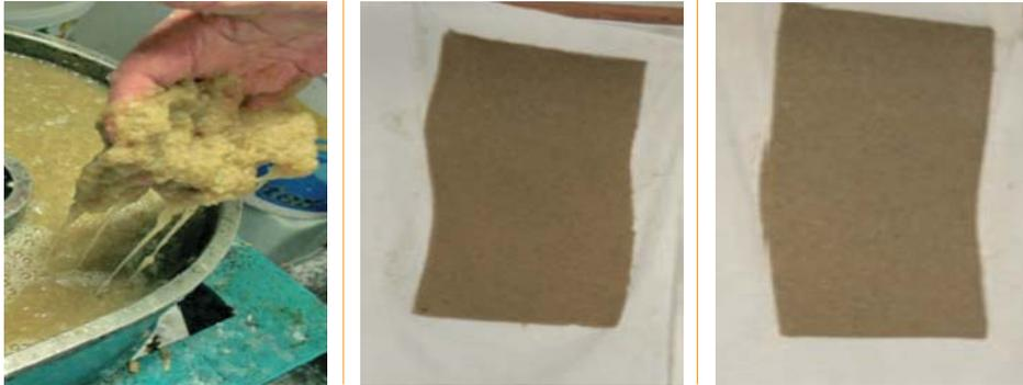
Water hyacinth pulp, non-absorbant fiber layer and absorbant fiber layer
