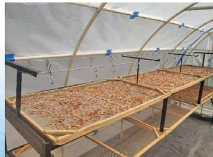
Solar tunnel dryer under loaded conditions
